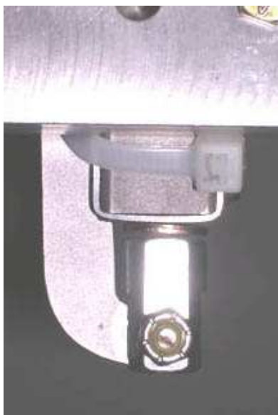
Figure 1.4: Clamp closed with zip tie
