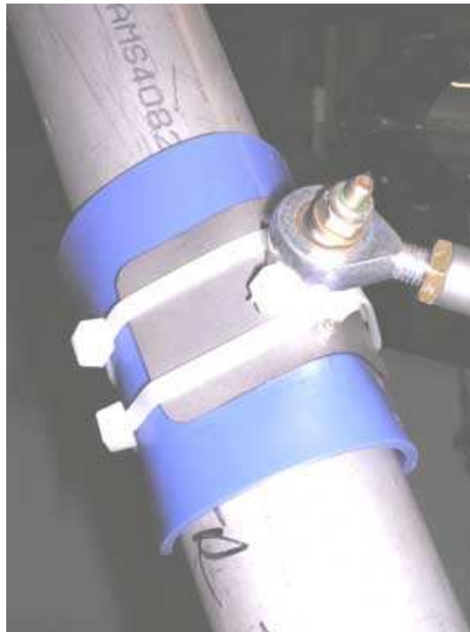
Figure 1.5: Proper Torque Arm attachment
